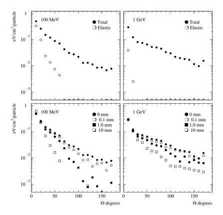
Fig. 3. Energy deposition in the polyethylene detectors as a function of angle with respect to the beam direction. Normalisation is to one particle incident on the  $30\,\mu\mathrm{m}$  wire.
