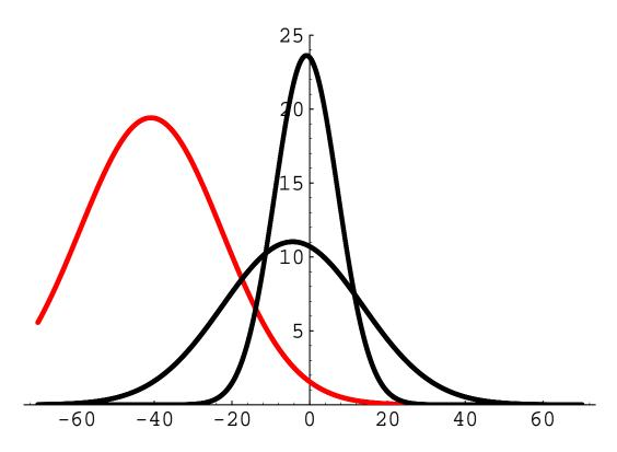
Fig. 8. In the centre of the figure the measured profiles for two beams with the same normalised emittance at two different energies, 100 MeV and 1.4 GeV, are shown. The wider profile at 100 MeV is slightly deformed due to geometrical effects. To the left in the figure a profile truncated at  $2\sigma$  from the profile centre is shown. The wire scanner software will for this profile deduce an emittance which is 20% smaller than the true emittance.
