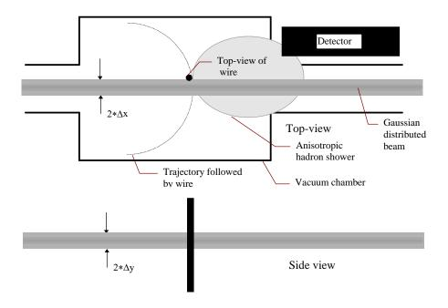
Fig. 1. Geometry of beam and wire
