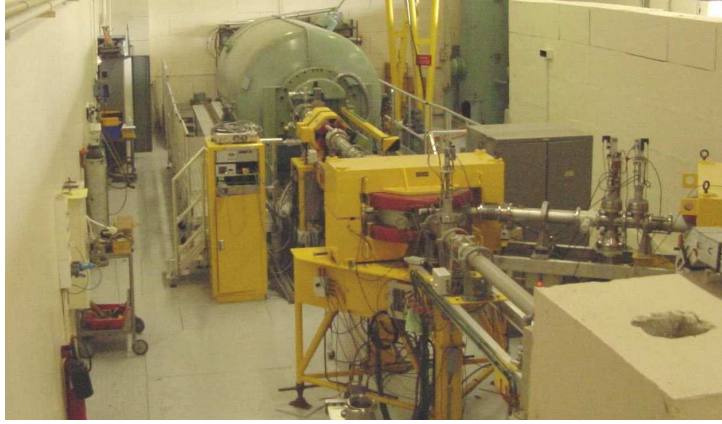
Figure 2.28: Photo of the Van de Graaff accelerator at CEA Bruyères-le-Châtel [72].
