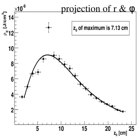
$\rho$ =k[wt<sup>a-1</sup>exp(-bt)+(1-w)l<sup>c-1</sup>exp(-dl)] w-"electromagneticity" of the cascade
