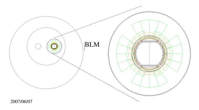
Coils are divided into small cells in (in  $r, \varphi, z$ ) which energy is measured.
