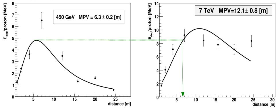
Signal in PMT scales with energy deposited in scintillators – there is a lot of signal at nominal luminosity – maximum 6-12 meters from WS, the signal level at 6 meters does not change with energy!
