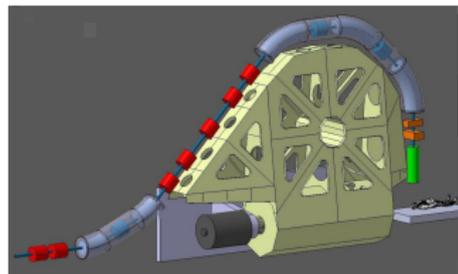
superconducting ion gantry,
