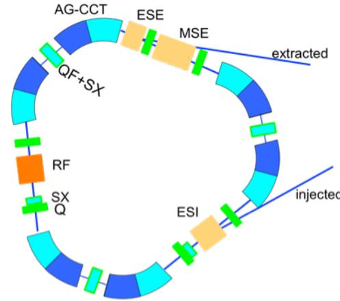
AG-CCT magnets allow periodic focusing while bending, reducing beta function (and beam size)
