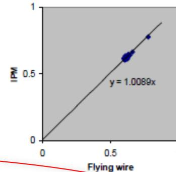
Comparison of vertical beam size from IPM and nearby Flying Wire. Tuning of abort cleaner timing had caused blow-up of certain bunches. From MAD lattice file, expect a 13% wider beam at Flying Wire. See ~1%.
