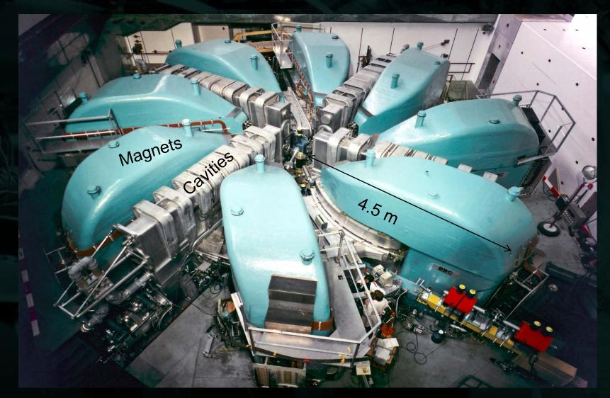
Accelerating protons from 72 MeV to 590 MeV, 1.3 MW beam power
