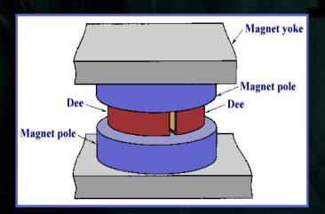
vacuum chamber: large narrow gap between 2 poles
