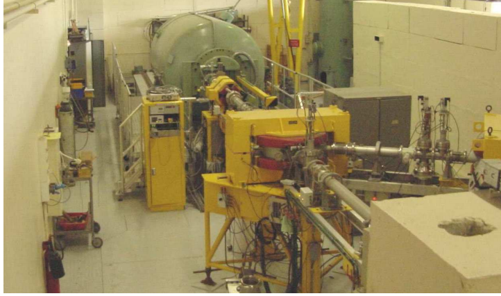
Figure 2.28: Photo of the Van de Graaff accelerator at CEA Bruyères-le-Châtel [71].
