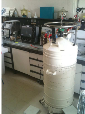
Figure 2.26: Photo of the experimental setup of the diamond test in LHe. The white Dewar filled with LHe is in the foreground and in the background.
