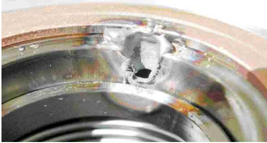
(a) Damaged inflicted to the beam pipe by the high-power electron beam of the ELBE accelerator [44].
