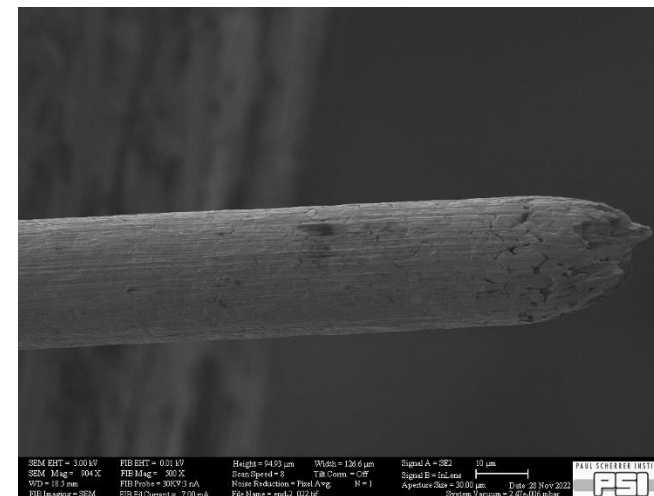
Broken Molybdenum wire with 25 \mu\text{m} of diameter
