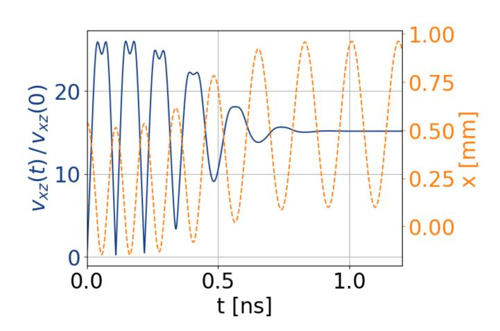
Example trajectory showing the oscillation of position and velocity in the electric field of the beam.
