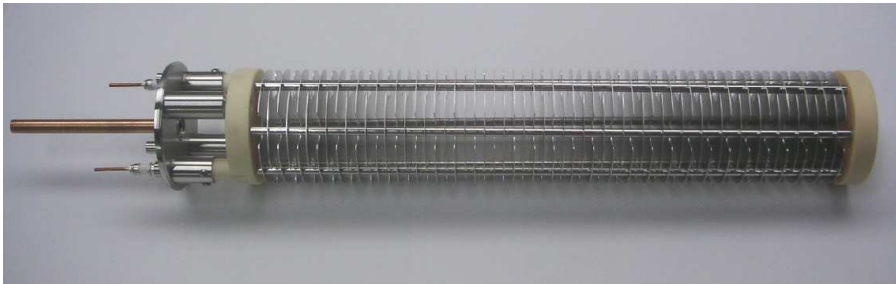
Figure 4.2: The LHC beam loss ionisation chamber.
