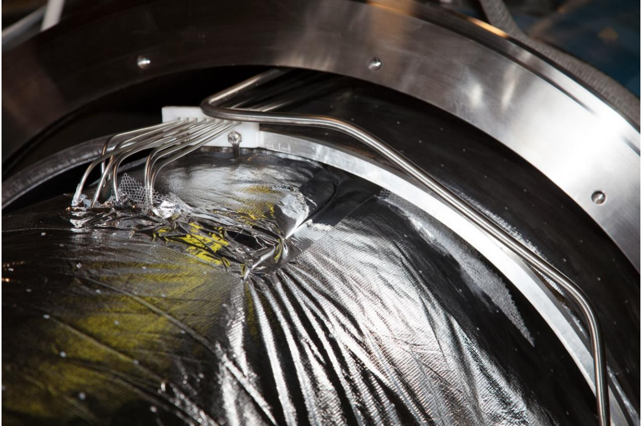
Figure 7: Routing of the cables through the last MLI layer.
