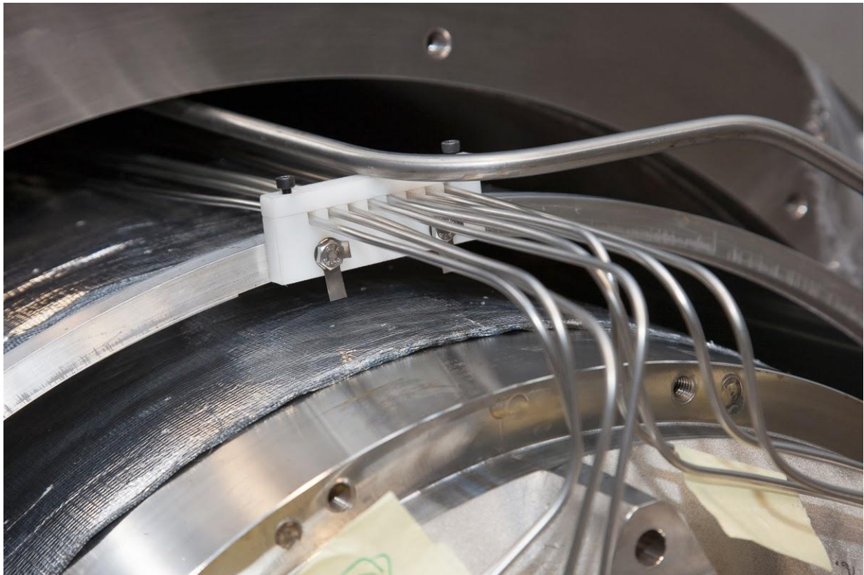
Figure 4: Cryogenic cable routing.
