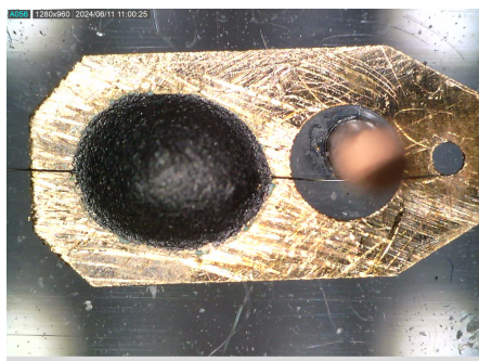
Figure 3: An image of the CuBe pad with glue and wire obtained using Dino-Lite AM7013MT digital microscope.
