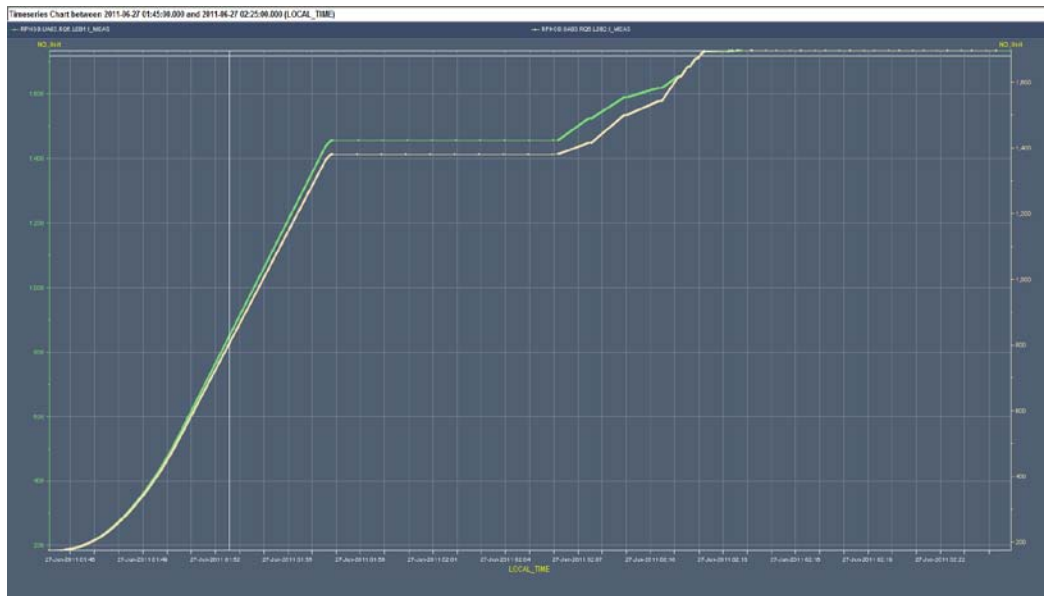
Figure 9 Current ramp in Q6.L8 magnet.
