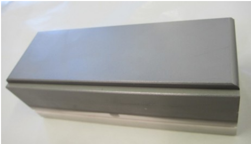
Figure 3: Boron nitride blocks with coating of 5 \mu\text{m} Ti, NEG, 2\mu\text{m} Cu and NEG before the bake-out.
