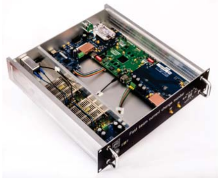
Figure 7: Picture of the operational FBCCM electronics box.
