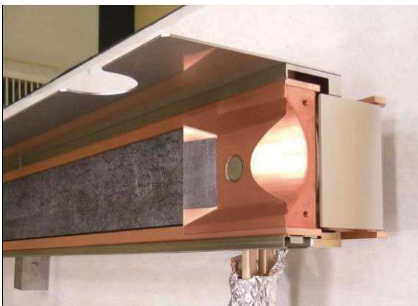
Figure 1: New TCSP carbon jaw with embedded BPM.
