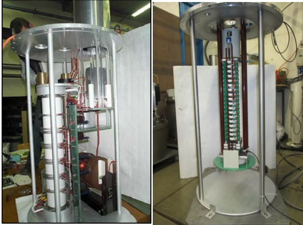
Figure 3: Thyatron (old system) left and thyristor (new system).
