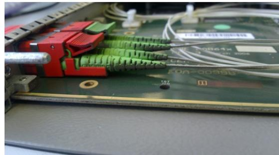
Figure 7: Example of dust accumulation on the optical link connectors.
