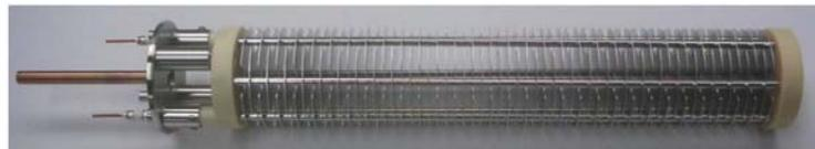
Figure 9: Inside view of a Beam Loss Monitor showing the electronic part at left and all the electrodes put in parallel at right.
