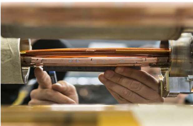
Fig 2: Marking the splice for R8/R16 measurements
