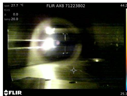
Figure 5: Carbon fibres glowing in visible spectrum due to excitation by RF field leaking from RF cavities.
