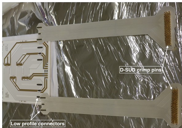
Figure 3. Left and right flexible cables with a blank chip carrier board.
