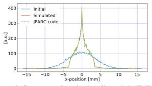
Figure 2: Comparison of simulated profiles with the JPARC code for the PS case (electron tracking).
