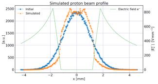
Figure 5: Simulated profile of the proton beam, integrated along y-direction. The bin size is  $30 \,\mu\text{m}$ . The (radial) electric field of the DC electron beam is indicated (dashed line).
