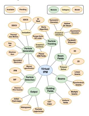
Figure 1: The different components (modules) of the simulation framework together with their corresponding models. Dashed ellipses indicate models in development.
