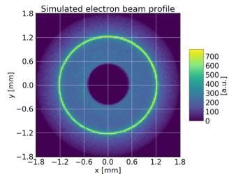
Figure 6: Simulated two-dimensional profile of the electron beam. The bin size is 30 µm. The original electron beam profile ranges from  $\sqrt{x^2 + y^2} = 1.2$  mm to 1.8 mm.
