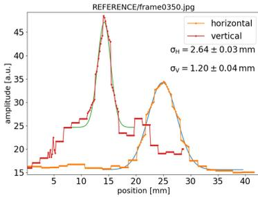
Figure 3: Example of beam profiles obtained with analog camera and a frame grabber on GTH2DFA screen.
