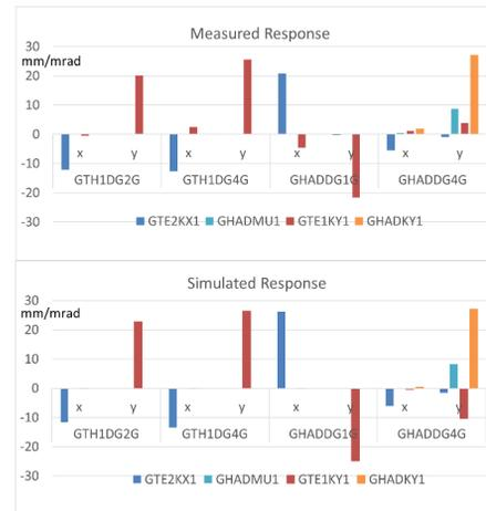
Figure 2: Measurement (upper) and modelling (bottom) of TRM.
